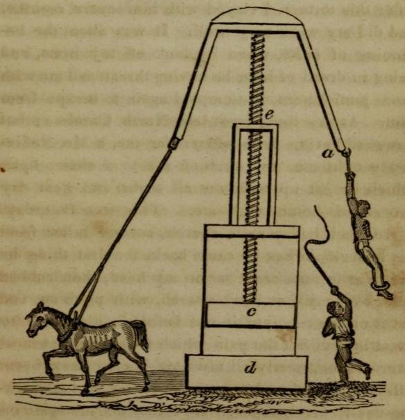
This is a machine used for packing and pressing cotton. By it he hung me up by the hands at letter a, a horse moving round the screw e, and carrying
